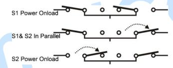
Fig. 6 Sync Transfer Diagram
