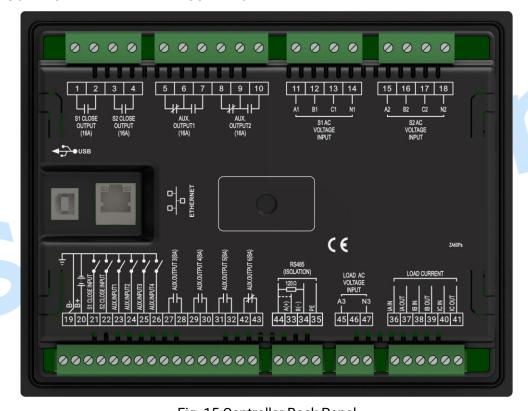
Fig. 15 Controller Back Panel
