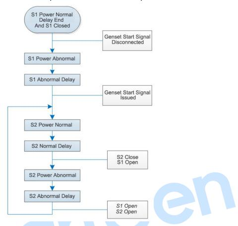
Fig. 8 Auto Transfer Non Restore Diagram (Mutual Backup Inactive)
