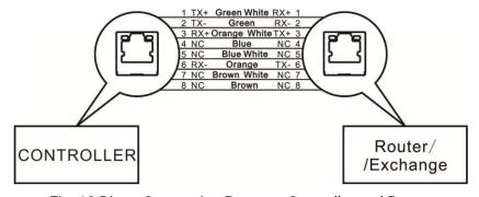
Fig. 13 Direct Connection Between Controller and Router
