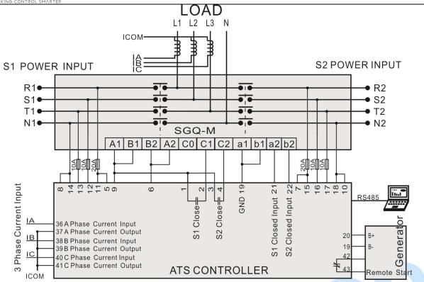
Fig. 20 SGQ-M Application Diagram
