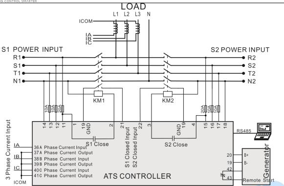
Fig. 23 Contactor Application Diagram
