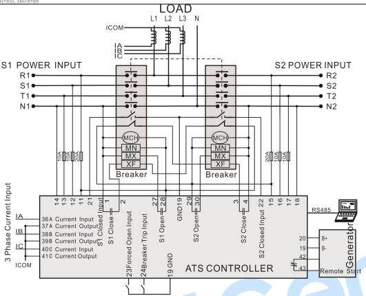
Fig. 24 Breaker Application Diagram
