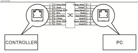
Fig. 14 Cross Connection Between Controller and PC
