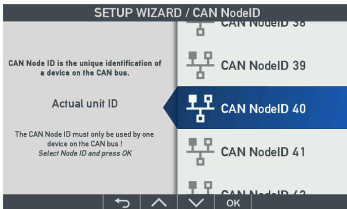
If the CAN bus/XDi-net is not used in your installation, please just press OK on the default CAN NodeID to continue.
