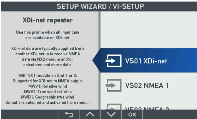
XDi-net data can come from the main XDi-N unit that is equipped with an NX2 NMEA extension module, where wind sensor data and other NMEA data are received and then distributed via XDi-net (CAN bus) to other XDi units on the same CAN bus.
