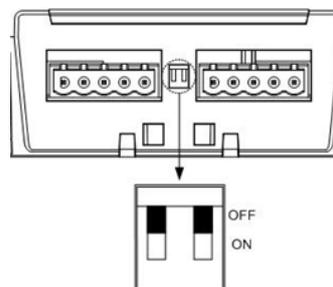
Terminate the RS-485 line from the sensor by shifting the red dill switch on the NX2 module to ON. See picture.
