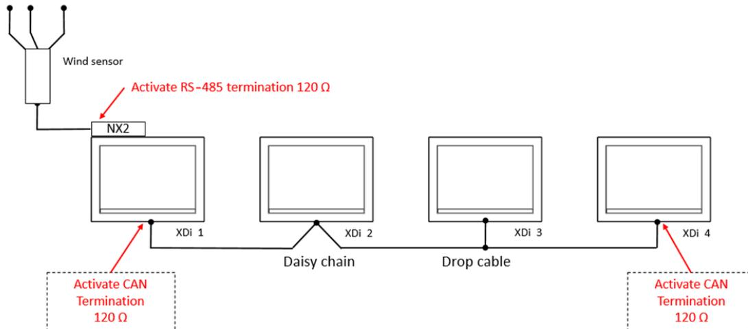
If the cable from the CAN angle transmitter is less than the max allowed drop cable length (10 m @125 kbps), then the CAN bus can be terminated using the internal termination in XDi 1 (left side), and the other termination can be made using the internal termination in XDi 3 (right side).
