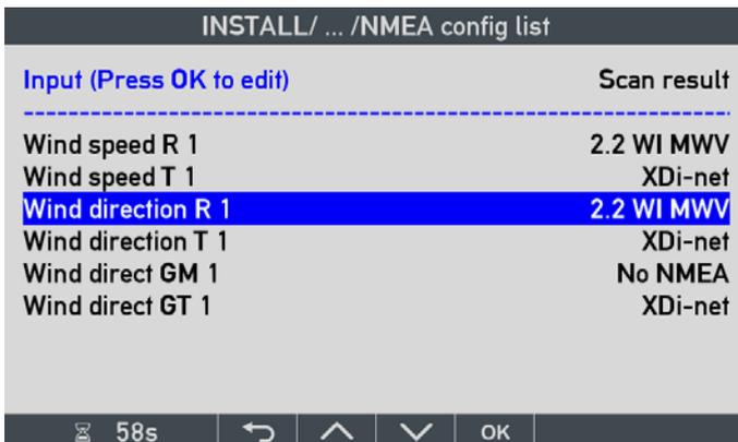
To correct the angle, select the "Wind direction R 1" (it is the relative wind direction instance 1).
