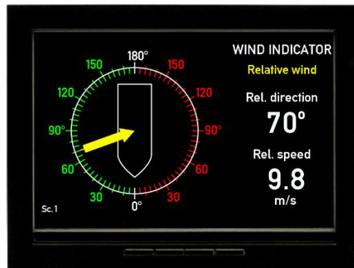
Relative wind indicator forward bridge (VI001)    Relative wind indicator aft bridge (VI002)
