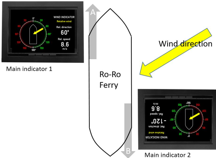
The sketch shows a ro-ro ferry with two main indicators placed on the two bridge locations. When the ferry is sailing in direction A, main indicator 1 is used for wind indication. When the ferry is sailing in direction B, which is now becoming the bow, main indicator 2 is used to show the wind direction. One of the indicators must be set up so that the wind direction input has an offset of 180°.
