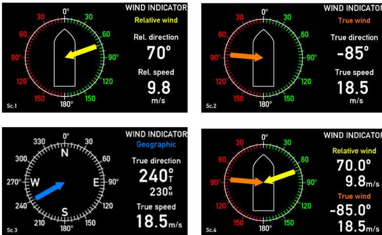
Toggle between the four screens showing: relative wind, true wind, geographic true wind and a combination of relative and true wind.
