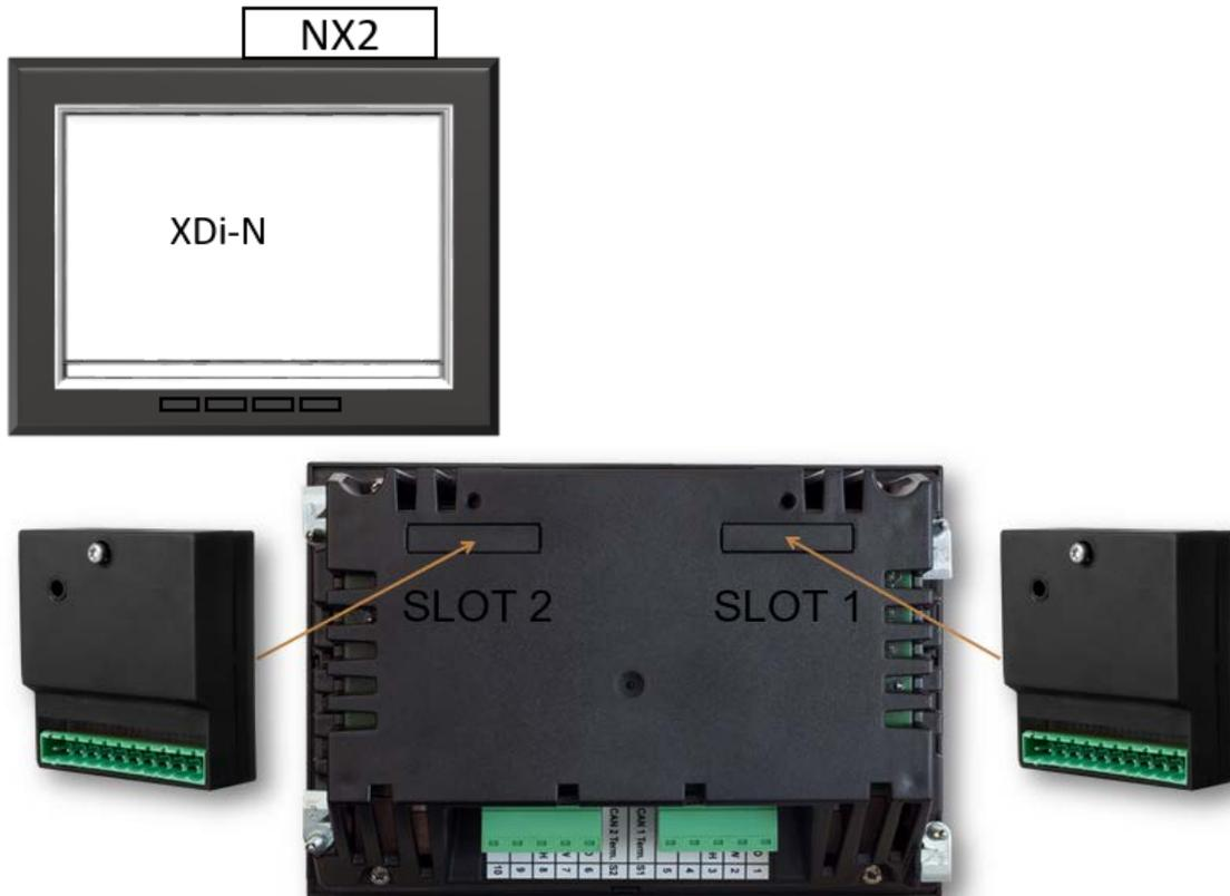
To present wind data from a wind sensor, an NX2 NMEA i/o extension module must be mounted to the rear of the XDi housing. The 3 NMEA inputs on the NX2 module enable the XDi-N to receive NMEA data from a wind sensor, true wind data from another system or speed and heading data to enable internal calculation of true wind data.
