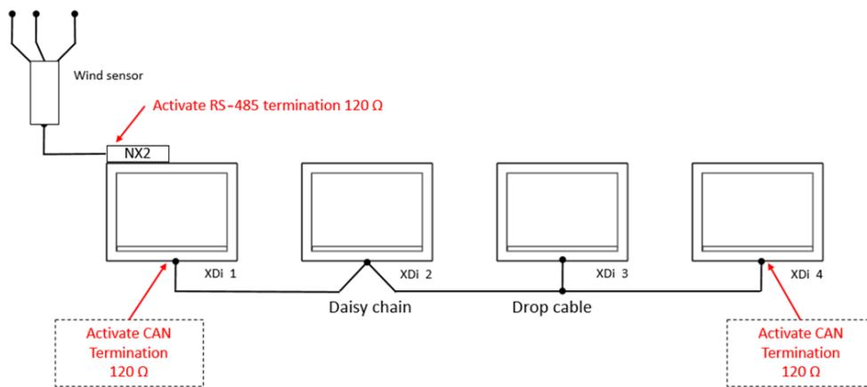
The standard terminal block, with a single row of 5 screw terminals, supplied as standard for the XDi-N, is most appropriate for drop cable connection. Daisy chaining will require two wires to be mounted in each terminal location.
