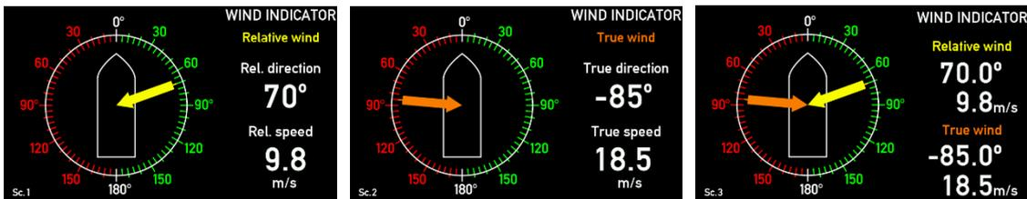
Toggle between the three screens showing: relative wind, true wind and a combination of relative and true wind.
