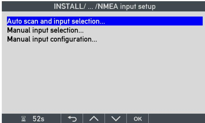
The “Manual input selection...” should first be used after the auto scan routine is performed. “Manual input configuration...” can be used to configure an NMEA input where no sentence is available when the input scanning is performed.
