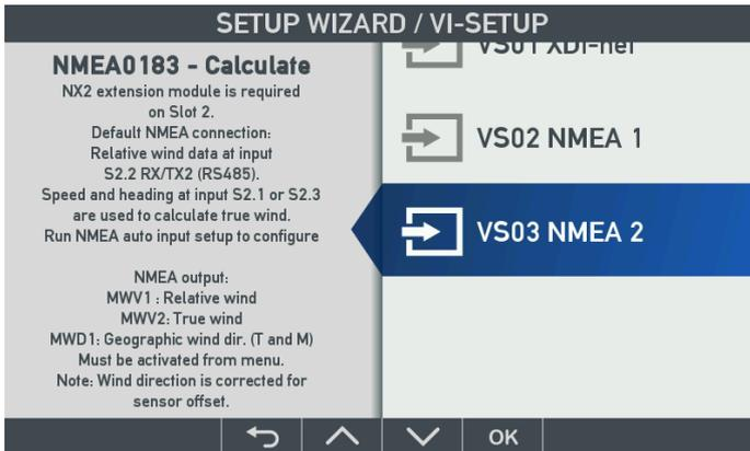
When using this profile, NMEA wind data can be retransmitted to the NMEA output (S2.1). From the XDi installation menu, a relative wind direction offset can later be inserted to compensate for a sensor misalignment.
