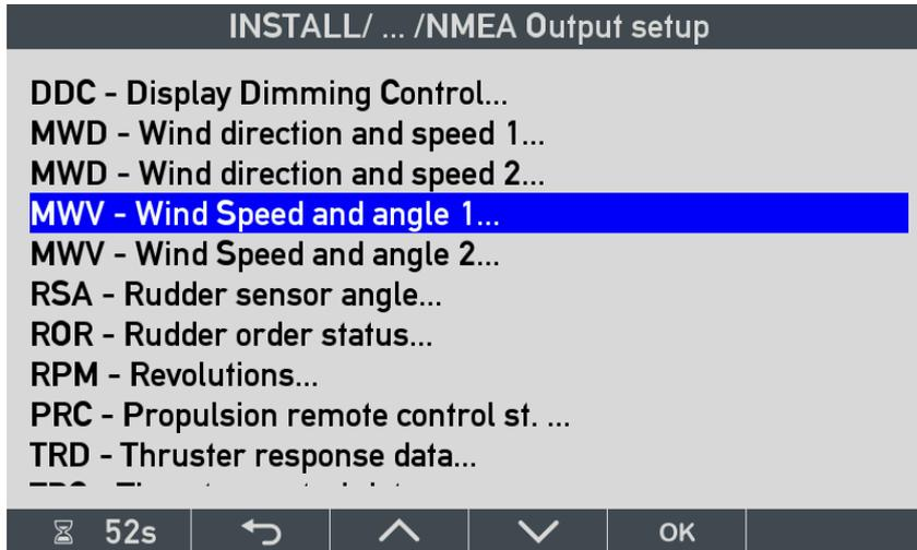
Please note that geographic true wind is contained in MWD not MWV. If geographic true wind speed and direction is to be transmitted on the NMEA output, select “MWD-Wind direction and speed 1” (instance 1).
