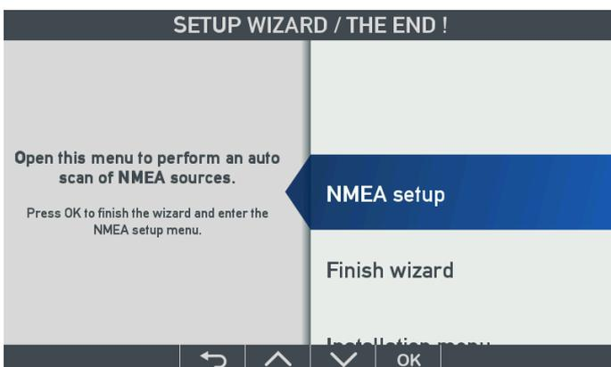
Before you push “OK”, it is a good idea to make sure that all relevant NMEA sensors and system devices are connected to the relevant NMEA inputs on NX2 and that they are powered up and transmitting data.
