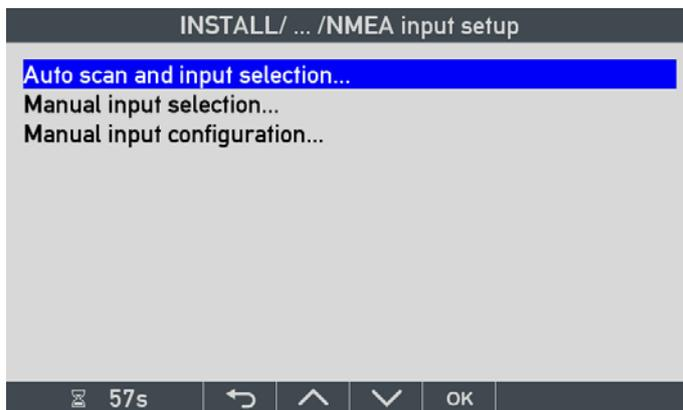
If a new NMEA source is added or a source is moved to another input port, you must run the auto scan again to update the list of available data sources.
