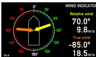
Use the left button on the front to toggle between the four screens showing: relative wind, true wind, geographic true wind and a combination of relative and true wind.
