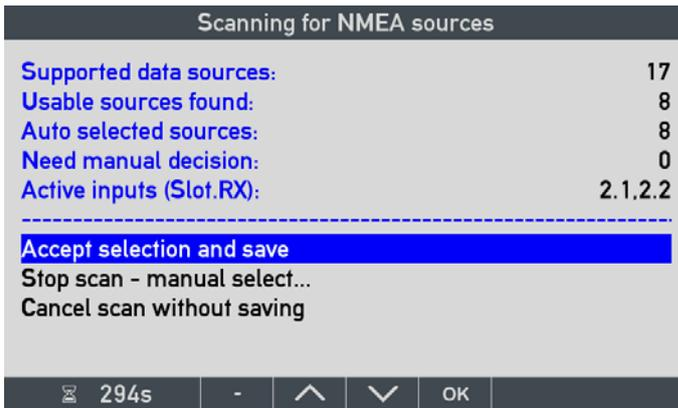
After a short period of time, the numbers in the right side will be stable. This means that no new data sources are detected.
