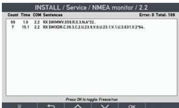
The NMEA monitor in the service menu is a powerful tool that makes it easy to see NMEA data received on the selected COM port. You can see data from a specific COM port, or from all COM ports simultaneously.
