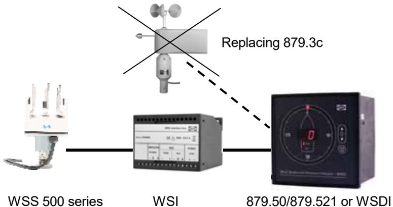
The special upgrade kit should be used when an existing 879.3c dynamic wind sensor is to be replaced with a new WSS 500 series sensor and connected to a display type 879.50/879.521 or WSDI. The interface box type WSI is needed to translate the RS-485 data signal from the WSS 500 series into a speed and direction TTL signal appropriate for the 879.50/879.521 or WSDI display.
