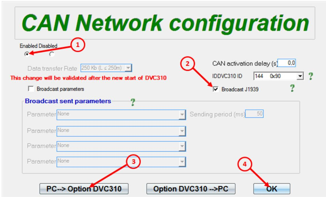
The buttons and check boxes marked with arrows must be checked. The regulators in the DVC 310 can now be tuned in.
