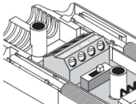
When the wiring is done, be aware whether the terminal resistor is ON or OFF. The terminal resistor can be set to on or off on the switch close to the terminals in the included CAN connector.
