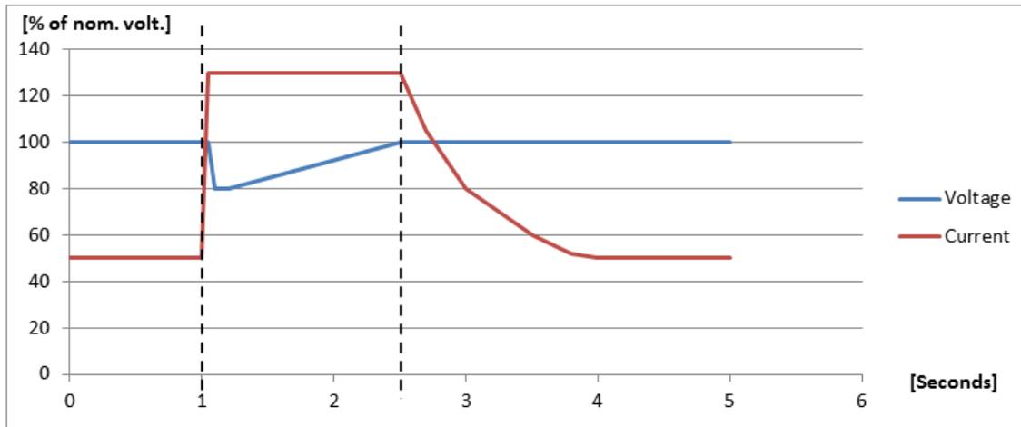
When the inductive load is turned on, the current will rise. The inductive motor starting function will limit the current to the predefined level set in parameter 7794. The AVR will change to have the current as set point and let the voltage drop. When the voltage reaches the nominal value again, the AVR will change to regulate with the voltage as set point again.
