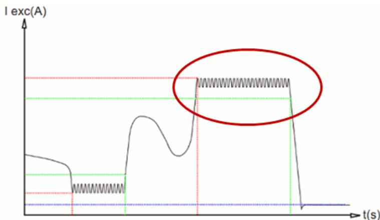
If the genset is supporting a very inductive load, the voltage on the alternator windings can be very high, even though nominal voltage is measured on the terminals. This protection contains three parameters, which can all be found in the EasyReg software.
