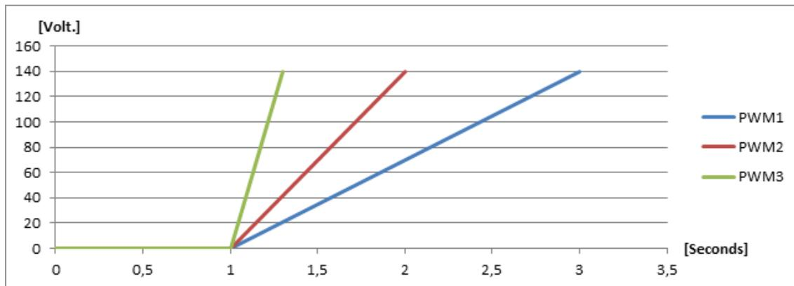
When the upper limit for the start-on threshold is changed, the start point for the soft-start is also changed. The upper limit for start-on threshold is always the start point for soft-start.
