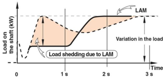
The graph above shows a comparison of the load on the shaft of the engine, with the LAM function enabled and disabled. When the LAM function drops the voltage, the torque on the shaft is lightened, which makes it possible for the engine to rise faster in RPM after a load impact. This also gives the possibility to steadily reach nominal values faster after the load impact, since the LAM function will give more stability.
