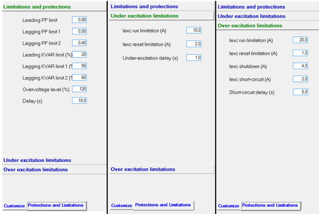
The three windows contain different settings. Some of them are used when the DVC 310 is interfaced with a Multi-line 2 unit. In the first window, only over-voltage and delay are used. None of the settings in the second window are used. In the third window, all settings are used. In the settings that are not used, a proper value must be entered. Proper values can be seen in mouse-over texts for each of them. Refer to the chapter "Protections" for a description of all protections.
