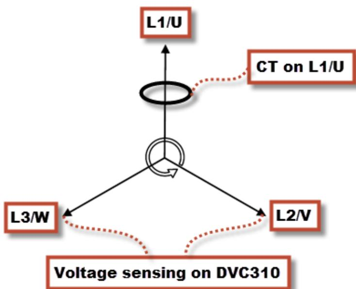
The DVC 310 will need to know the correction in degrees between the voltage sensing and the current measurement. In this example, the correction will be 90 degrees, which can be set in the EasyReg software.
