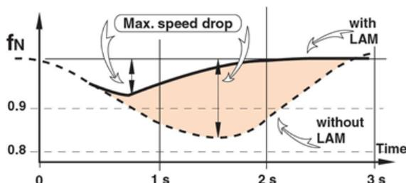
The graph above shows that with the LAM function, the frequency will rise and stabilise faster after a big load impact. This is because the LAM function will drop the voltage and by this lower the torque on the engine.
