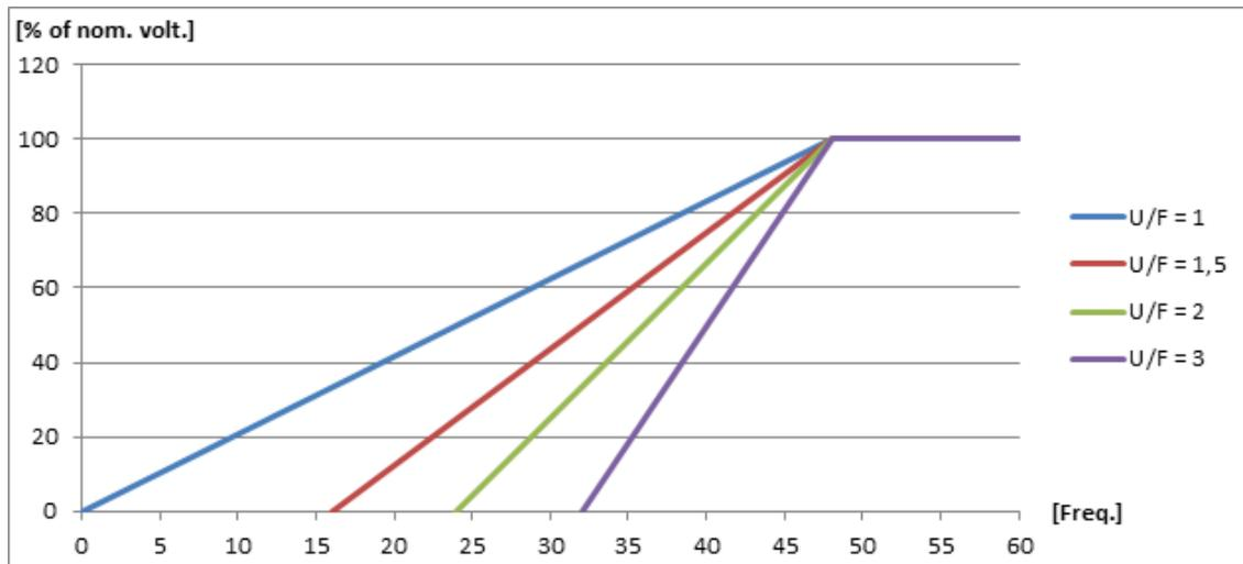
The knee point determines when the knee function is active. When the frequency goes below the knee point, the U/f law defines a temporary voltage set point for the AVR.
