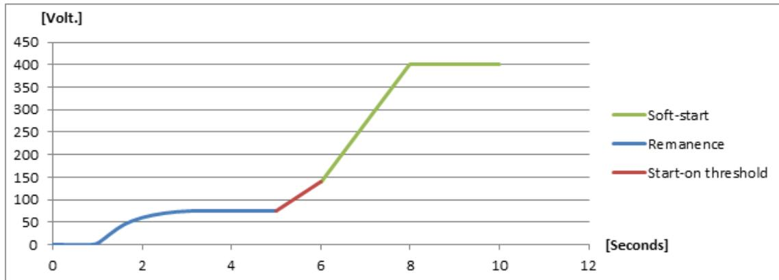
The soft-start timer in CBE is not the same as the soft-start timer in normal start, but the start-on threshold parameters are the same as in the normal start. Having different settings for the soft-start gives the possibility to have for example a more aggressive excitation ramp for CBE sequences. The timer for the soft-start in CBE is located in parameter 2262. Note that this timer is different from the one in normal start.
