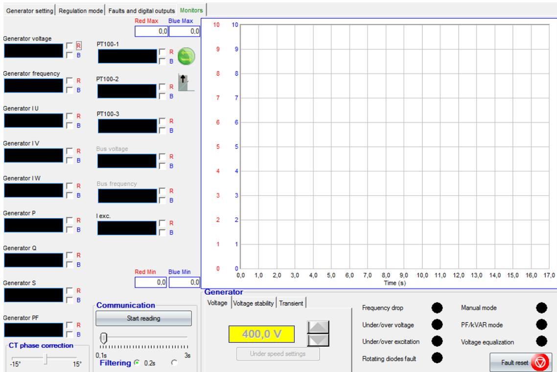
In this window it is possible to trend for example the voltage and the frequency at the same time. The monitor is limited to trending max. two different things at a time. The trending window can be helpful when tuning in the regulators. A transient test can be started in the monitor window. When the transient test is started, the voltage set point will be changed. The set points for the transient test are set by the user.
