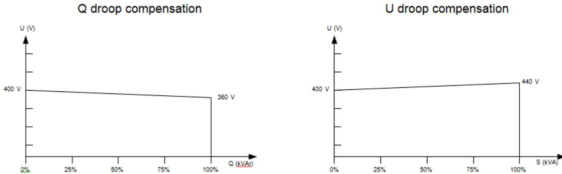
The droop compensation decides how much the voltage is allowed to droop if the regulation is turned off in the Multi-line 2 unit. The regulation can be turned off by setting the Multi-line 2 unit into MANUAL. The regulation can also be off if the CAN bus cables should break. With the droop, it is possible to give the AVR a set point for the voltage if an error in the CAN bus lines should occur. This makes it possible for the genset to share the reactive load when no interfacing is available.
