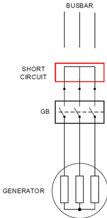
2. Choose Dry alternator mode in menu 6071. Start the genset in semi-auto mode and close the GB. When the windings are dried out, open the GB and stop the genset.
