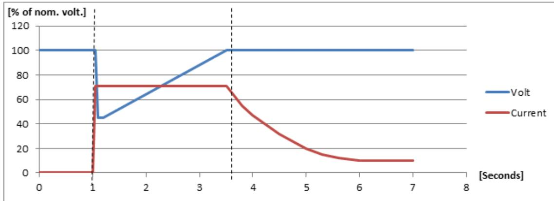
The first dotted line shows when the generator breaker closes. The second dotted line shows when the transformer magnetisation function will be deactivated. (5 % below the current limitation set point set in menu 7793).
