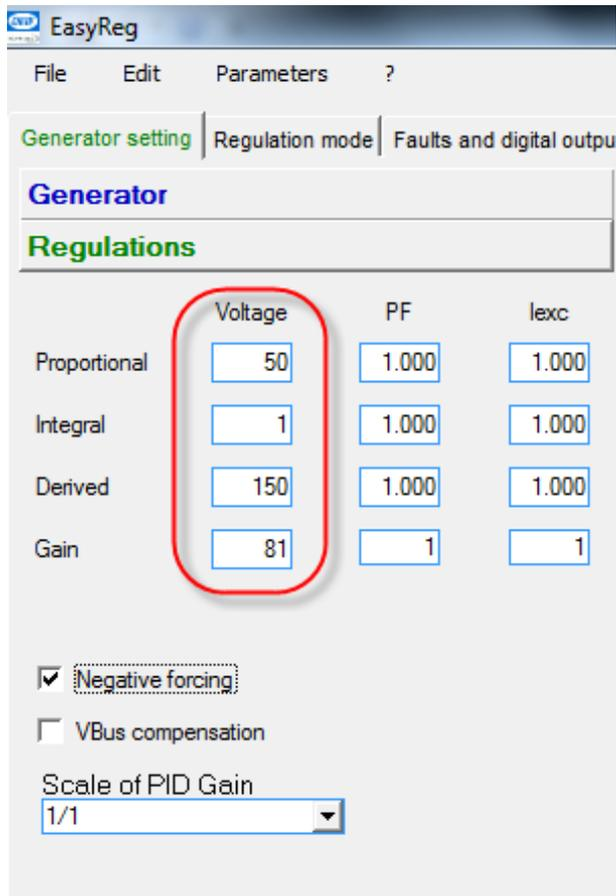
The EasyReg software has a feature called transient test, which is really useful for tuning in the voltage regulators.
