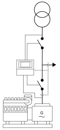
**Automatic mains failure (AMF)**
